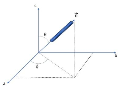
A hexagonal crystal is cut in a thin rod with a direction at an angle  $\theta$  = 54° with the c-axis, and the angle between the a-axis and the projection of the direction of the rod in the ab-plane is  $\phi$  = 48°. A current is flowing along the rod. Find the electrical resistivity of the rod when the components of the resistivity tensor are  $\rho_{11} = 5 \cdot 10^{-8} \Omega cm$  and  $\rho_{33} = 3 \cdot 10^{-8} \Omega cm$ Select one alternative
