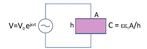
A dielectric solid has a homogeneous complex relative dielectric constant  $\epsilon = \epsilon'_r - \epsilon''_r$ . Consider the circuit as shown in the figure above. Numerical values are as follows: The voltage amplitude  $V_0 = 25V$ , the voltage angular frequency  $\omega = 10000 \text{ s}^{-1}$ , the capacitor area A = 10 cm<sup>2</sup>, the separation of the capacitor plates h = 1 mm, and the relative dielectric constant  $\epsilon = 2 + j0.5$ .
