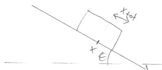
Endring i potentiell energi:  $\Delta U = -mgh = -mg x_{\text{tot}} \sin \theta$
