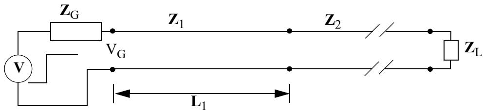
A voltage step of 6V is sent from a source to a transmission line with real impedance  $Z_1$  and length  $L_1$  as shown in the figure above. The first transmission line is connected to another transmission line of real impedance  $Z_2$ . At the end of the second transmission line is a load of impedance  $Z_L$ .
