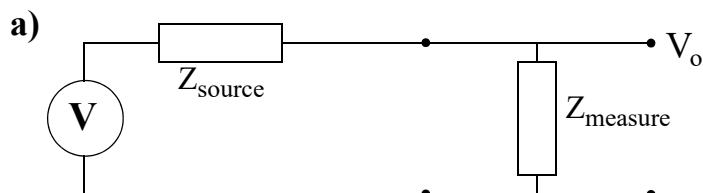
The figure above shows an equivalent circuit for a voltage source and a measurement circuit.
