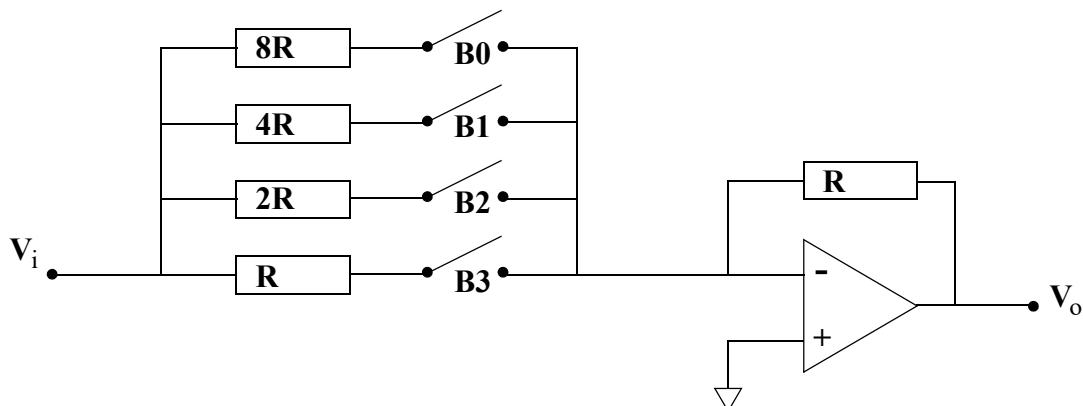
The figure above shows a circuit consisting of an operational amplifier and resistors of values  $R$ ,  $2R$ ,  $4R$  and  $8R$  as indicated. In addition there are switches  $B_0$ ,  $B_1$ ,  $B_2$  and  $B_3$ . The input voltage is  $V_i$  and the output voltage is  $V_o$ .
