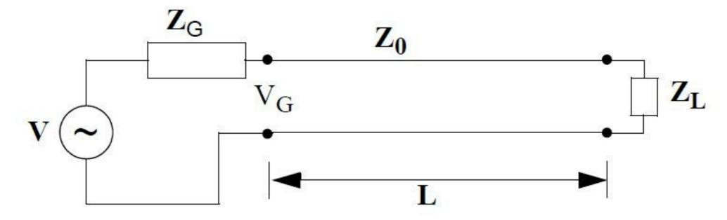
A high frequency voltage signal is transmitted to a transmission line of length L as shown in the figure.  $Z_G$  and  $Z_L$  are the impedances of the generator and load; respectively.  $Z_0$  is the characteristic impedance of the transmission line. The inductance and capacitance per length of the transmission line are L = 350nH/m and C = 80pF/m. The transmission line may be assumed to be loss-less.
