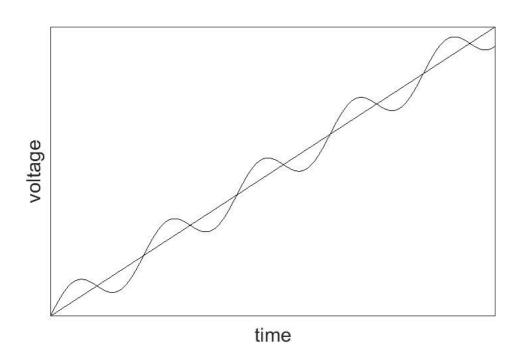
A linear voltage signal has superimposed a noise signal that may be approximated by a sinusoidal function. The total voltage becomes  $V(t) = \alpha t + Asin(\omega t)$ . Estimate the quantization noise of the signal when A = 4V.
