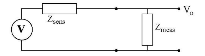
The figure above show an equivalent circuit for a voltage source and a measurement circuit. The impedance for the source  $Z_{sens}=50\Omega$ .
