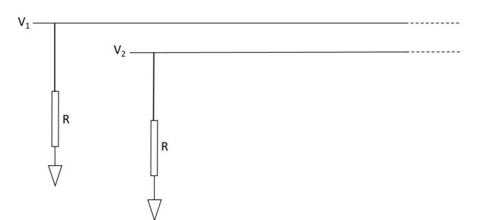
Two long signal cables are placed next to each other as shown in the figure. Both cables have a finite resistance to ground. There is a stray capacitance between the two cables.
