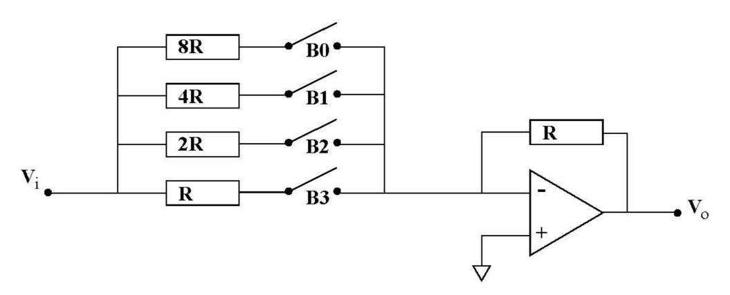
The figure above shows a circuit consisting of an ideal operational amplifier, resistors and switches B0 to B3.  $V_i = 8V$  and  $V_o$  are the input and output voltages, respectively, and the value of R = 100 $\Omega$ .
