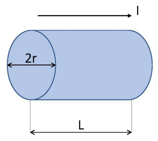
A current flows through a resistor shaped as a cylinder of resistivity  $\rho$ , length **L** and radius **r**, as shown in the figure above.
