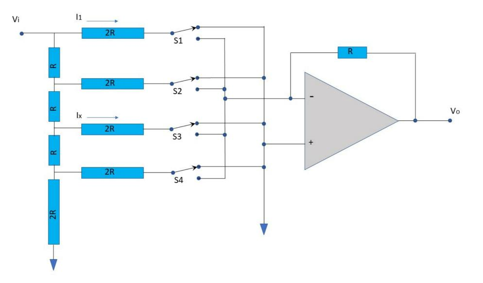
The DAC circuit shown above consists of resistors with resistances R and 2R as indicated, switches S1 to S4, and an ideal operational amplifier. The reference voltage is  $V_i$  and the output voltage is  $V_o$ . Currents  $I_1$  and  $I_x$  are indicated in the figure.
