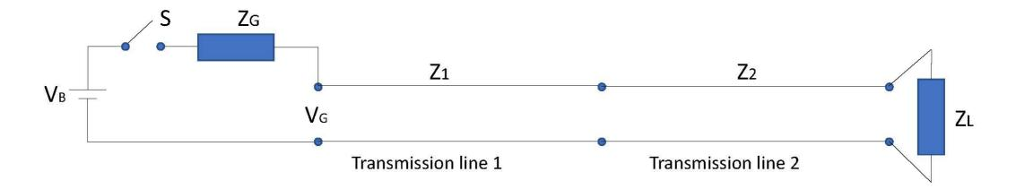
A battery of voltage  $V_B$  and a switch **S** generates a step voltage  $V_G = 6V$  at the start of transmission line 1. Impedances are given by  $Z_G = 75\Omega$  and  $Z_1 = 75\Omega$ . What is the voltage  $\boldsymbol{V}_{\boldsymbol{B}}$  of the battery ?
