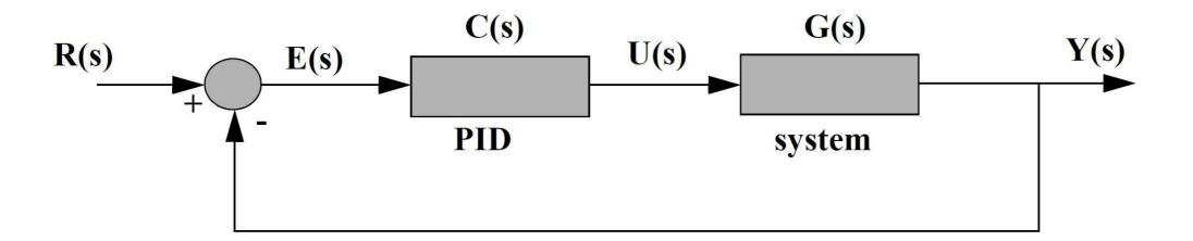
A PID regulated system is shown in the figure above.
