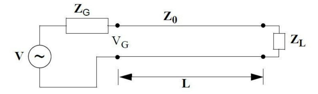
The figure above shows a generator circuit that transmit a high frequency signal on a transmission line of characteristic impedance  $Z_0$ . At the end of the line is a load impedance  $Z_L = 1000\Omega - i300\Omega$ .
