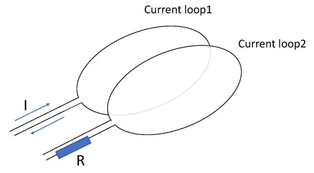
An **AC** current **I=2A** of frequency **f=500Hz** in **loop1** induces a voltage and current in nearby **loop2** as shown in the figure. The mutual inductance of the current loops is  $M=0.5\mu$ H.
