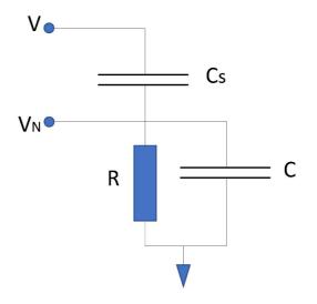
The input circuit of an amplifier consists of a  $R = 200\Omega$  resistor in parallel with a C = 100pF capacitor as shown in the figure above. A power line of frequency f = 650Hz and peak to peak voltage V = 500V is coupled to the input circuit by a stray capacitance  $C_s = 60pF$ , which results in a noise voltage of  $V_N$  at the input of the amplifier.
