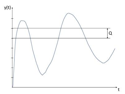
An analogue signal as shown in the figure above is to be digitized. The resolution of the ADC is **Q= 2mV**. Assuming uniform distribution of deviation from the analogue signal, what is the value of the quantization error of the digitized signal?
