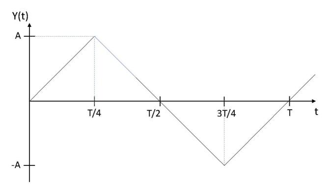
One period of a periodic signal is shown in the figure above. The maximum value of the signal is A=4V, and the period is T.
