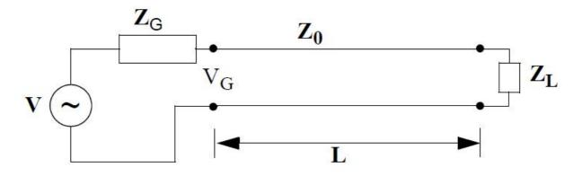
The figure above shows a generator circuit that transmit a high frequency signal on a transmission line of characteristic impedance  $Z_0 = 75\Omega$ . At the end of the line is a load impedance  $Z_L = 450\Omega + i200\Omega$ .
