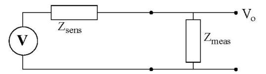
An AC voltage source has amplitude V = 100V and output impedance  $Z_{sens} = (100 + j50)\Omega$ . The input of an amplifier circuit is described by the input impedance  $Z_{meas} = (500 - j100)\Omega$ . See figure above.
