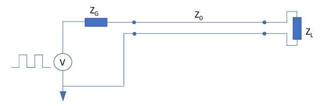
A high frequency pulse train enters a transmission line as shown in the figure. At the end of the transmission line is a load. The line impedance  $Z_0 = 75\Omega$ , and the load impedance consists of a parallel coupling of resistor  $R = 200\Omega$  and a capacitor  $C = 0.4\mu F$ . The frequency of the pulse train is f = 1000Hz.
