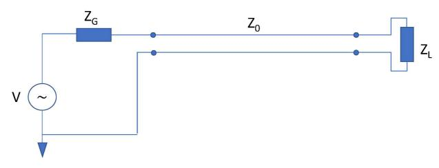
A voltage signal of angular frequency  $\omega = 1 \cdot 10^8 s^{-1}$  is incident on a transmission line of characteristic line impedance  $Z_0$ , as shown in the figure above. The inductance and capacitance per unit length of the transmission line are L = 250nH/m and C = 100pF/m, respectively. Assume loss-less transmission line. The load impedance is  $Z_L = 200\Omega$ .
