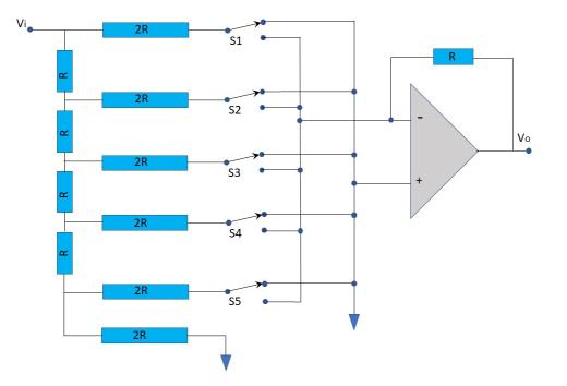
The DAC circuit shown above consists of resistors with resistances R and 2R as indicated, switches S1 to S5, and an ideal operational amplifier. The reference voltage is  $V_i = 5V$  and the output voltage is  $V_o$ .
