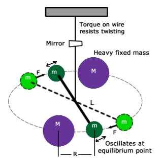
The gravitational constant  $G = 2\pi^2 \frac{x \cdot R^2 \cdot L}{T^2 \cdot Y \cdot M}$  may be estimated from the Cavendish experiment as illustrated above. Here **Y** is the distance from mirror to ruler, **x** is the distance on the ruler which measures the angle of rotation, **R** is the distance between masses **M** and **m**, **L** is the length of the torsion arm, and **T** is the period of oscillation.
