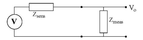
The figure above show an equivalent circuit for a voltage source and a measurement circuit. The impedance for the source  $Z_{sens} = (200 + 50i)\Omega$ .
