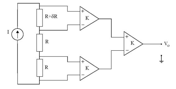
The above figure shows an "Anderson loop" circuit having three differential amplifiers of gain K and resistors of values R and R+ $\delta$ R and a current source of current I. What is the output voltage V<sub>o</sub> for K = 8, I=0.1A, R = 1000 $\Omega$ , and  $\delta R$ = 0.1 $\Omega$ ?
