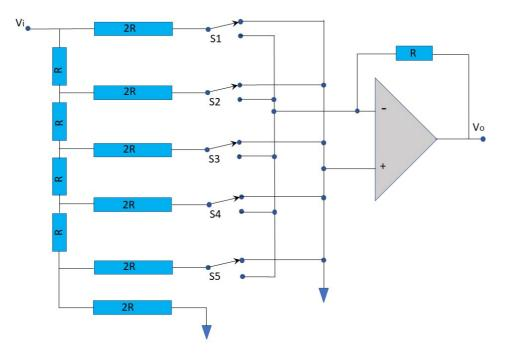
The DAC circuit shown above consists of resistors with resistances R and 2R as indicated, switches S1 to S5, and an ideal operational amplifier. The reference voltage is  $V_i = 8V$  and the output voltage is  $V_o$ .
