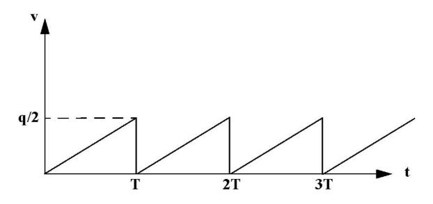
A noise signal v of period T and amplitude q/2 (as shown in the figure above) is superposed on a voltage signal V. What is the RMS value of the noise signal (quantization noise)? Use for the resolution q = 0.01V and calculate a number.
