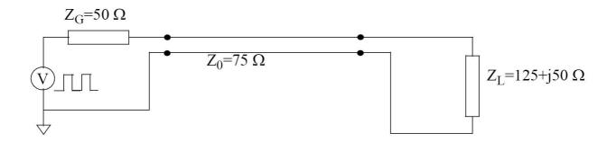
A high frequency pulse train enters a transmission line as shown in the figure. At the end of the transmission line is a complex load that consists of a serial coupling of a resistor and a solenoid. Find the reflection coefficients at the load. Give the answer in amplitude and phase angle. Assume loss-less transmission line.
