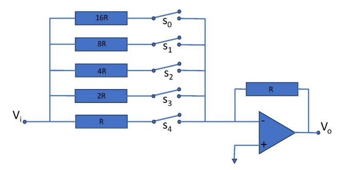
The DAC shown in the figure above consists of an ideal operational amplifier, resistors and switches. The reference voltage V<sub>i</sub> = +4V, and R = 100  $\Omega$ .
