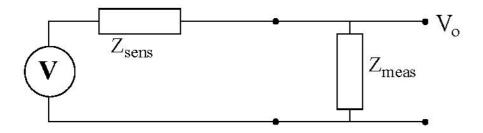
The figure above show an equivalent circuit for a voltage source and a measurement circuit. The impedance for the source  $Z_{sens} = 50 + j20 \Omega$ .
