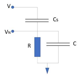
The input circuit of an amplifier can be considered to consist of a  $R = 10M\Omega$  resistor in parallel with a C = 100pF capacitor as shown in the figure above. A power line of frequency f = 50Hz and peak to peak voltage V = 320V results in a noise voltage of  $V_N = 1V$  at the input of the amplifier due to capacitive coupling.
