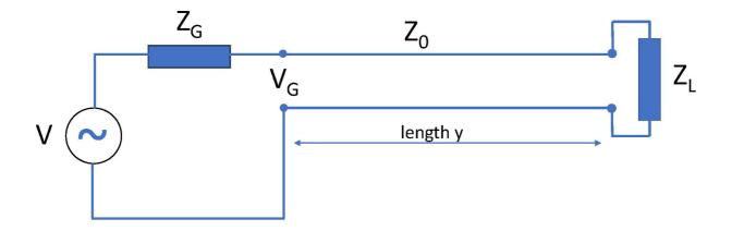
A high frequency voltage signal of angular frequency  $\omega = 1 \cdot 10^9 s^{-1}$  is transmitted from a source to a transmission line of length y, as shown in the figure above.
