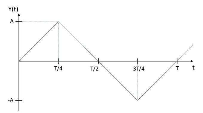
One period of a periodic signal is shown in the figure above. The maximum value of the signal is A=6V, and the period is T.
