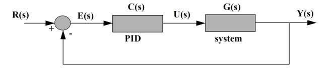
A PID regulated system is shown in the figure above.
