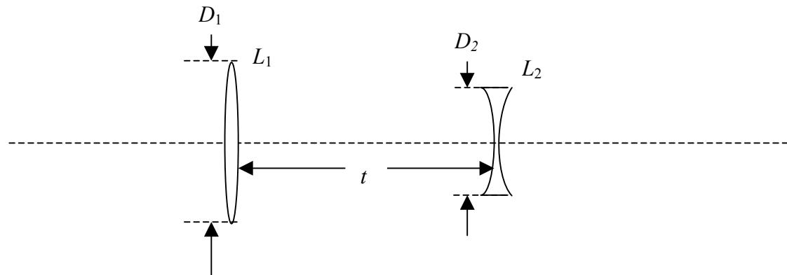
The figure shows a composite system made up of two thin lenses in air ( $n = 1$ ): One positive lens  $L_1$  and one negative lens  $L_2$ , with focal lengths, respectively,  $f_1 = 15 \text{ cm}$  and  $f_2 = -3 \text{ cm}$ , that are separated by a distance  $t$ .
