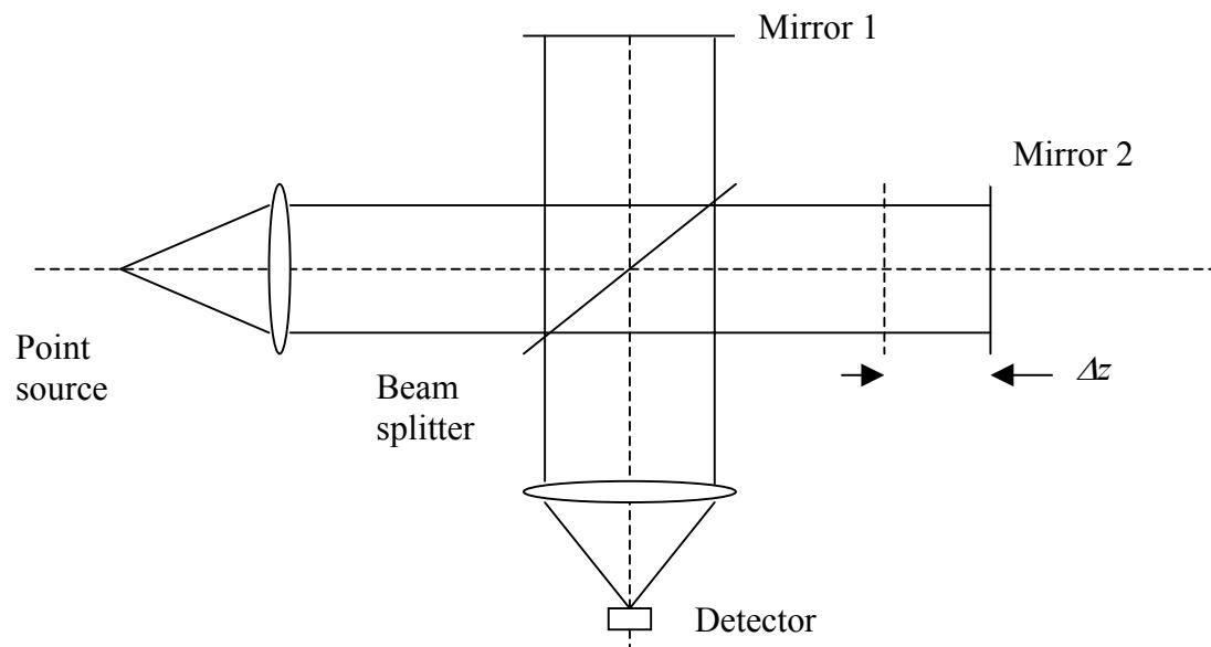
The figure illustrates a Michelson-interferometer with collimated point-source illumination. We assume that the two interfering waves have equal intensities, and that the interferometer is perfectly aligned. The detected intensity is a function of the path-length difference  $s = 2\Delta z$ , where  $\Delta z$  is the displacement of mirror 2 from the position with zero path-length difference.
