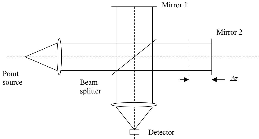
The figure illustrates a Michelson-interferometer with collimated point-source illumination. We assume that the two interfering waves have equal intensities, and that the interferometer is perfectly aligned. The detected intensity is a function of the path-length difference  $s = 2\Delta z$ , where  $\Delta z$  is the displacement of mirror 2 from the position with zero path-length difference.
