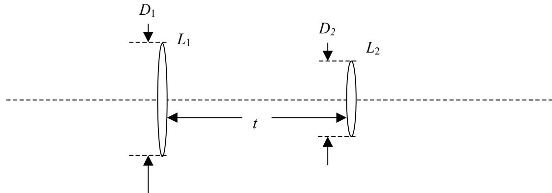
The figure shows a composite system made up of two thin lenses in air ( $n = 1$ ),  $L_1$  and  $L_2$ , with focal lengths, respectively,  $f_1 = 30 \text{ cm}$  and  $f_2 = 5 \text{ cm}$ , that are separated by a distance  $t = f_1 + f_2 = 35 \text{ cm}$ . The ray transfer is limited by the two lens holders with diameters, respectively,  $D_1 = 8 \text{ cm}$  and  $D_2 = 2 \text{ cm}$ .
