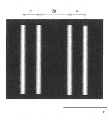
A 1D diffraction grating consists of 4 identical lines with Gaussian transmission function. The spacings between the lines are a, 2a, and a, as illustrated in the sketch above.
