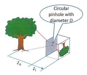
A pinhole camera is illustrated in the figure above. Pinhole cameras are historically the first kind of cameras. In this task, the pinhole camera has a circular aperture of diameter D and a fixed distance  $z_i = 100$  mm from the aperture to the image plane. There is a square-shaped area detector located in the image plane having side lengths of 70 mm. We assume  $z_0 >> z_i$ . The wave length  $\lambda$  of the incoming light can be approximated to 550 nm.
