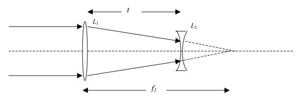
For the object point on axis we now have the situation illustrated in the figure above and, from the given dimensions and the results above, we immediately see that  $\underline{L_1}$  is the aperture stop. Since we only have two stops,  $\underline{L_2}$  is the field stop.
