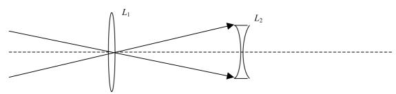
For the bundle of chief-rays that limits the angular field of view, we have the situation illustrated above. The angular diameter of the field of view is therefore equal to the angle subtended by  $L_2$  at  $L_1$ :  $\frac{D_2}{t} = \frac{1}{12.5} \frac{180^0}{\pi} = 4.594^0$ .
