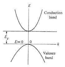
Assume that we have a semiconductor with a direct gap  $E_g$  as shown in the figure. The valence band has a parabolic E(k) with hole mass  $m_h$  and the conduction band is also of parabolic form with electron mass  $m_e$ . Assume that the matrix element M for an optical transition near k=0 is constant. Show that the joint density of states for the system is  $\sim \sqrt{\hbar\omega - E_g}$  and that  $\epsilon_2$  thus is of the form
