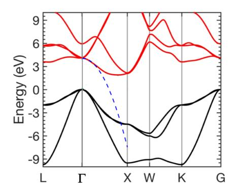
The blue broken line is a parabola fitted to the lowest-energy conduction branch near the  $\Gamma$ -point along the  $\Gamma X$ -path. The energy is defined to be zero at the top of the valence band. The direct bandgap at  $\Gamma$  is 4.1 eV. For fcc structures, the X-point is at  $2\pi/a$ .
