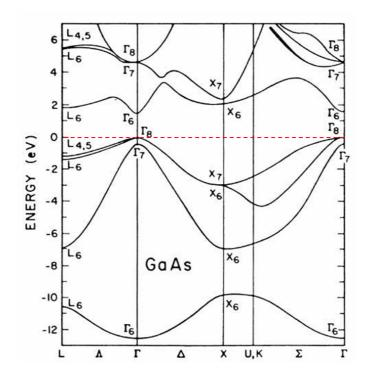
The above figure shows the band structure of intrinsic GaAs. The broken red line indicates the top of the valence band (with energy defined to be zero).
