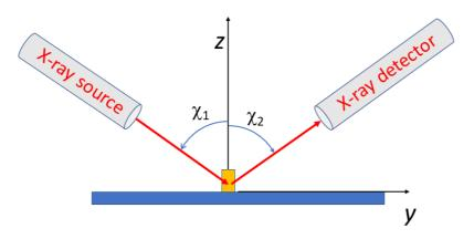
The experimenter wants to measure the diffracted intensity from the *001* Bragg peak. Which of the statements is correct?
