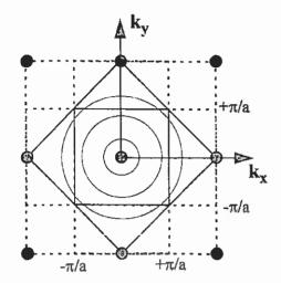
The figure shows a two dimensional reciprocal lattice. The circles represent constant energy contours in the free electron model.
