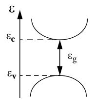
The figure shows a schematic representation of the direct band gap semiconductor InP. The semiconductor is undoped. The band gap is 1.42 eV. The effective masses are:  $m_e^* = 0.07m_e$ ,  $m_h^* = 0.05m_e$  The temperature T = 300 K.
