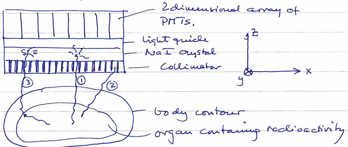
Each PMT is assigned an address  $x_i, y_j$  in the two dimensional image plane xy.
