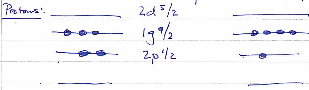
A proton is raised from the  $2p^{1/2}$  state to the  $1g^{9/2}$  state, thus giving an even number of protons in  $1g^{9/2}$  with no spin contribution (due to pairing). Spin and parity will be determined by the odd proton in  $2p^{1/2}$ , i.e.  $I = 1/2$ , parity  $(-1)^e = (-1)^1 = -1$ , i.e.  $^{1/2^-}$  g.r.o.d.
