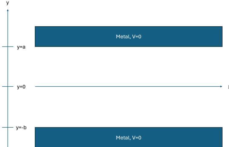
Figure 1: A sheet of surface charge at y = 0 is between two grounded metal conductors at y = a and y = -b . Although not shown, the system is supposed to be infinitely homogenous in the x and z directions. At y = 0 , there is a surface charge density \sigma(x, t) that may depend on the spatial coordinate x and the time t .
