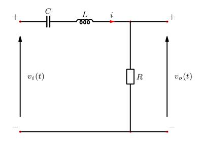
**A.** Write a differential equation which relates the output  $v_o(t)$  with the input  $v_i(t)$  for this system. (5p)
