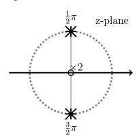
**Answer:** Signal described by this diagram as a transfer functions with poles at  $z = \pm j = e^{\pm j\pi/2}$ . Using the formula derived above we can write:
