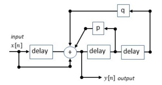
Find the values p and q of the amplifiers in order to generate the output sequence  $y[n] = 0.5^n$  using the digital impulse response as the input signal. (Only give the answers !)
