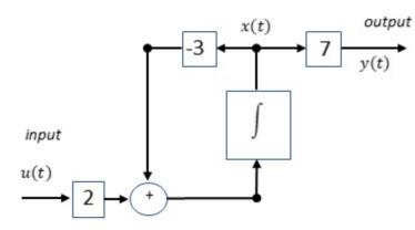
y(t) is the output, u(t) is the input, and the variable x(t) is defining the initial state.
