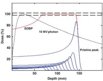
Red line: Spread out Bragg peak in a typically therapeutic radiation distribution. The depth dose plot of a 10 MV photon beam is provided for comparison
