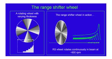
The Bragg peak is expanded in the depth of the tumour by using a rotating wheel with varying thickness to modulate the energy to obtain beams of lower intensity and shorter range producing the SOBP distribution
