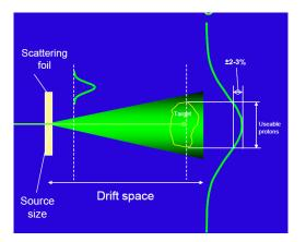
Spread out the beam laterally using a scattering foil. Broadening the beam Gaussian typically 20 cm
