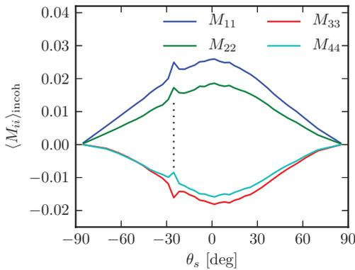
FIG. 3. (Color online) The incoherent contribution to the diagonal Mueller matrix elements,  $\langle M_{ii} \rangle_{\text{incoh}}$ , in the plane of incidence (parameters as in Fig. 2). The vertical dotted line indicates the backscattering direction. The lines, from top to bottom, correspond to  $i = 1, 2, 4$  and 3.
