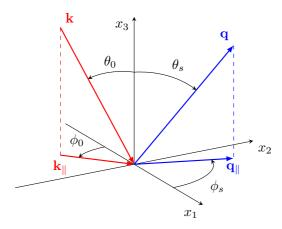
FIG. 1. A sketch of the scattering geometry assumed in this work. The figure also shows the coordinate system used, angles of incidence  $(\theta_0, \phi_0)$  and scattering  $(\theta_s, \phi_s)$ , and the corresponding lateral wave vectors  $\mathbf{k}_{\parallel}$  and  $\mathbf{q}_{\parallel}$ , respectively.
