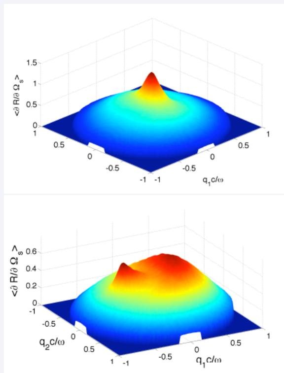
Comparison of the Perfect Conductor and Metal case for  $\lambda = 1\mu\text{m}$
