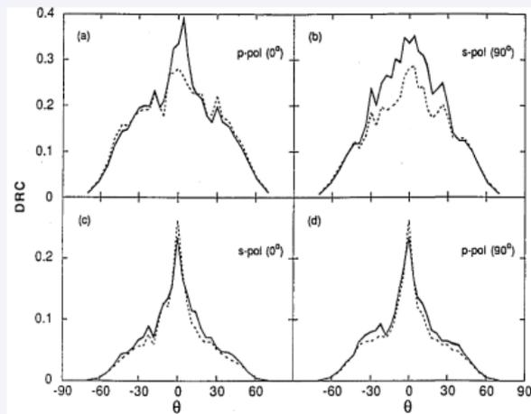
The contribution to the mean differential reflection coefficient from the incoherent component of the scattered light for scattering from a metal surface ( $\delta = \lambda$ ,  $a = 2\lambda$  with  $\lambda = 1\mu\text{m}$ ).
