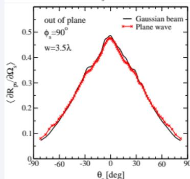
At least for the parameters used in the numerical simulations, there seems to be only limited effects of the edges when using a plane incident wave.
