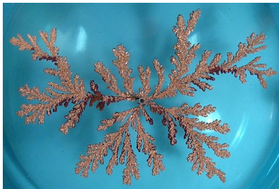
A DLA cluster grown from a copper sulfate solution in an electrodeposition cell
