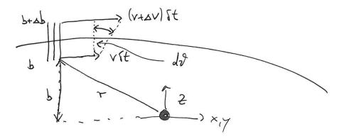
Figure 2.1: The difference velocity v(r)=c/n(r) of light-rays leads according to Hyggen's principle to the deflection of light.
