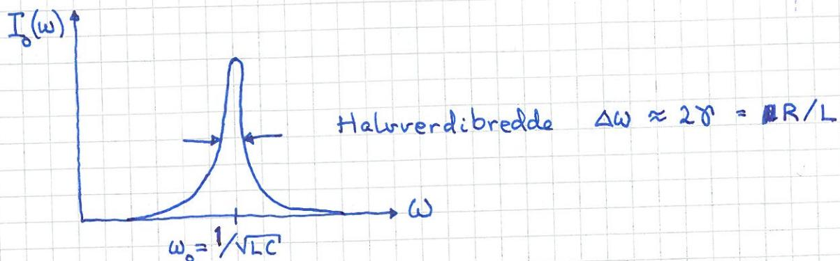
$$\text{Eks (LAB): } L = 22 \text{ mH}, \quad C = 0.15 \mu\text{F}, \quad R = 20 \Omega$$
