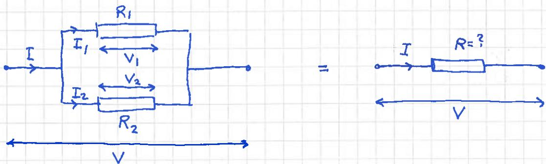
$$I = I_1 + I_2 = \frac{V_1}{R_1} + \frac{V_2}{R_2} = V \left( \frac{1}{R_1} + \frac{1}{R_2} \right) ; \quad I = V \cdot \frac{1}{R}$$
