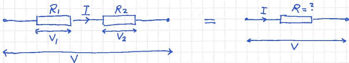
$$V = V_1 + V_2 = R_1 I + R_2 I = (R_1 + R_2) I ; \quad V = R I$$
