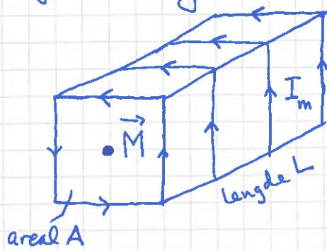
$\vec{M} \stackrel{\text{def}}{=} \text{magn. dipolmoment pr volumenhet}:$
