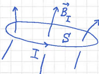
$$\phi = \int_S \vec{B}_I \cdot d\vec{A} = \underbrace{\int_S \left\{ \frac{\mu_0 I}{4\pi} \oint \frac{d\vec{s} \times \hat{r}}{r^2} \right\} \cdot d\vec{A}}_{= \vec{B}_I} \quad (\text{Biot-Savart, s. 109})$$
