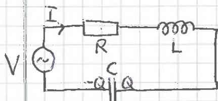
$$K2: V_0 \sin \omega t - RI - L\dot{I} - \frac{Q}{C} = 0$$
