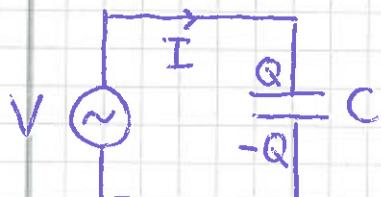
$$K2: V_0 \sin \omega t - \frac{Q}{C} = 0$$
