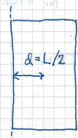
$$\begin{aligned} I &= I_0 + M \cdot \left(\frac{L}{2}\right)^2 \\ &= \frac{1}{3} M L^2 \end{aligned}$$
