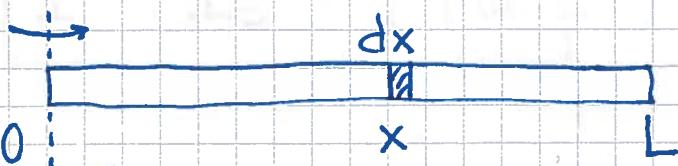
$$I = \int_0^L x^2 M dx / L = \underline{\underline{\frac{1}{3} ML^2}} \quad (\text{oppgis ikke})$$
