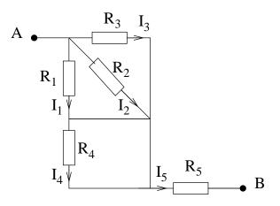
a) Determine the total resistance R between the points A and B, i.e.: Determine the resistance R in the equivalent circuit in the following figure:
