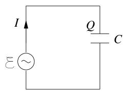
Find the charge Q(t) on the capacitor, and also the current I(t) in the circuit. Sketch  $\mathcal{E}(t)$  and I(t) between t = 0 and  $t = T = 2\pi/\omega$ .
