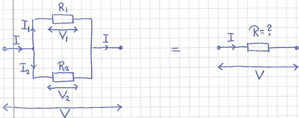
Lik spenning over de to motstandene;  $V_1 = V_2 = V$
