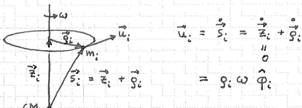
$$\Rightarrow \frac{1}{2} \sum_i m_i u_i^2 = \frac{1}{2} \left\{ \sum_i m_i g_i^2 \right\} \omega^2 = \frac{1}{2} I_o \omega^2$$
