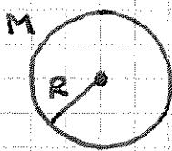
$$I_0 = \int_{\text{ring}} g^2 dm = R^2 \int_{\text{ring}} dm = MR^2$$
