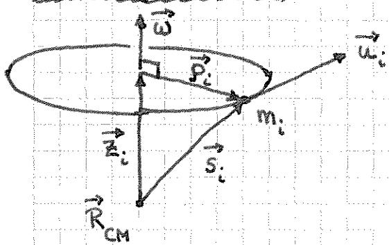
$$\begin{aligned} \vec{r}_i &= \vec{R}_{CM} + \vec{s}_i \\ \vec{v}_i &= \vec{V} + \vec{u}_i \\ (\vec{r}_i) &= \vec{R}_{CM} + \vec{s}_i \end{aligned}$$
