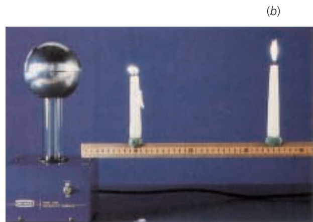
FIGURE 22-23 (a) A plot of E_r versus r for a spherical-shell charge distribution. The electric field is discontinuous at r = R , where there is a surface charge of density \sigma . (b) The decrease in E_r over distance due to a charged spherical shell is evident by the effect of the field on the flames of these two candles. The spherical shell at the left (part of a Van de Graaff generator, a device that is discussed in Chapter 24) carries a large negative charge that attracts the positive ions in the nearby candle flame. The flame at right, which is much farther away, is not noticeably affected.
