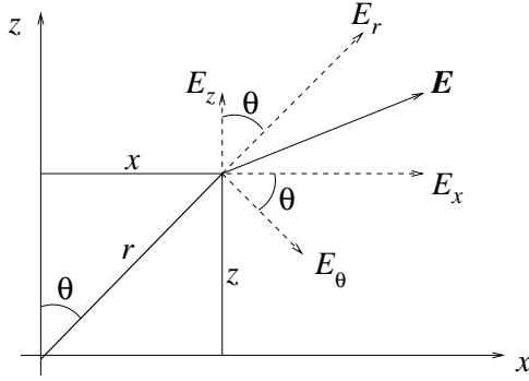
Both  $E_r$  and  $E_\theta$  have components in the  $x$  direction, and the total  $x$  component of the field must be the sum of these two. Looking at the figure, we have
