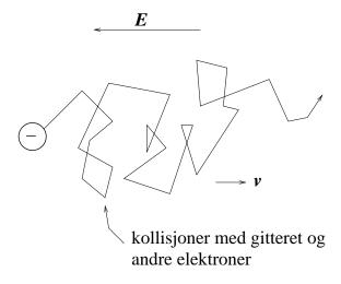
Mean drift velocity along -E: v
