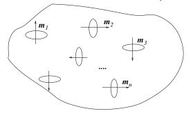
Earlier in this course, we have studied electric dipoles with dipole moment p, and we have seen how these are subject to a torque  $\tau = p \times E$  in an electric field E, so that they are aligned along the external field. We have seen that this is relevant for understanding how dielectric materials behave in an electric field, because a dielectric consists of atomic or molecular electric dipoles, i.e., atoms or molecules with electric dipole moment p.
