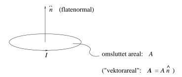
Magnetic dipole moment (for *plane* current loop):
