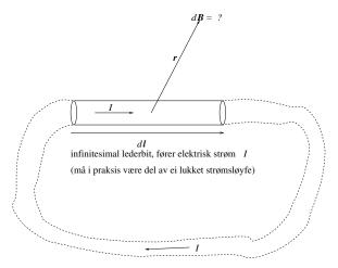
The contribution  $d\mathbf{B}$  to the magnetic field in the point in distance  $\mathbf{r}$  from the wire element  $d\mathbf{l}$ , when the wire carries a stationary (i.e. time independent) current I, is
