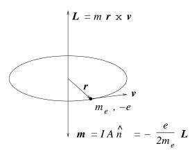
Electrons (and protons and neutrons etc) also have "inner angular momentum", i.e. spin S. Classical picture of spin for electron: Rotating charged sphere. Classically, we expect contribution
