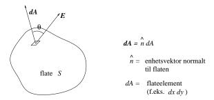
The surface S is an arbitrary "thought" or "chosen" surface in space. The electric field "exists" in the region where the surface S is "located". ( $\mathbf{E}$  may be zero, or nonzero.) The surface S is
