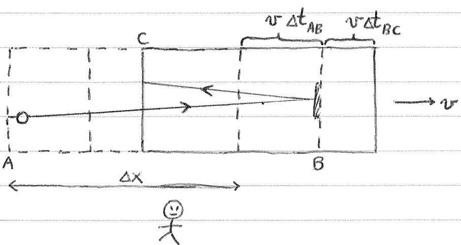
$$\Delta t_{AB} = \frac{\Delta x}{c} + \frac{v \Delta t_{AB}}{c}, \quad \Delta t_{BC} = \frac{\Delta x}{c} - \frac{v \Delta t_{BC}}{c}$$
