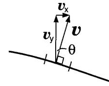
Fig. 2. Geometry of an element of string moving perpendicularly to its local direction.  $v$  is the actual velocity vector of the string element in this case, and it has components  $v_x$  and  $v_y$  in the  $x$  and  $y$  directions, respectively. The angle between  $v_y$  and  $v$  is  $\theta$ .
