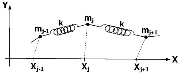
Fig. 1. Schematic of our model of an ideal string: a lattice of point masses joined by massless, linearly elastic springs with spring constants  $k$ . As a wave passes, the point masses  $m_j$  move from their equilibrium positions  $(X_{j,0})$  to  $(x_j(t), y_j(t))$ . In its undisturbed state,  $|X_{j\pm 1} - X_j| = l > a$ , where  $a$  is the relaxed length of each spring, so that a string under tension is modelled.
