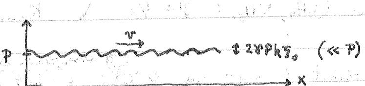
$$\text{Intensiteten: } I = \frac{1}{2} \rho \omega^2 \vec{s}_0^2 v \quad (\text{W/m}^2)$$
