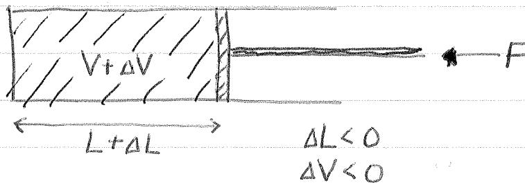
$$\frac{F}{A} = -B \frac{\frac{\Delta L}{L}}{\Delta L} = -B \frac{\Delta V}{V}$$
