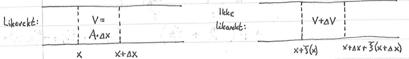
$$\Delta V = A \{ \vec{s}(x + \Delta x) - \vec{s}(x) \} \approx A \left\{ \vec{s}(x) + \Delta x \frac{\partial \vec{s}}{\partial x} - \vec{s}(x) \right\} = A \Delta x \frac{\partial \vec{s}}{\partial x}$$
