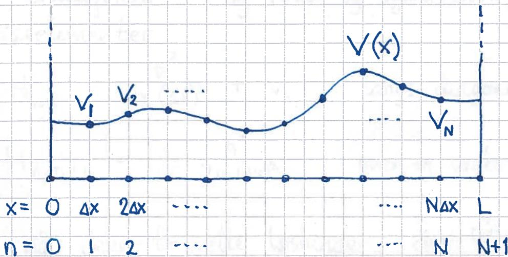
$$\Rightarrow x_n = n \cdot \Delta x, \quad V_n = V(x_n); \quad n = 0, 1, \dots, N, N+1$$
