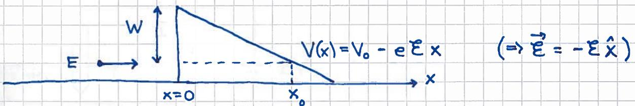
$$V(x_0) = E \Rightarrow V_0 - eEx_0 = V_0 - W \Rightarrow x_0 = W/eE$$
