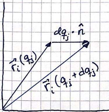
$$\begin{aligned} \frac{\partial \vec{r}_i}{\partial q_j} &= \lim_{dq_j \rightarrow 0} \frac{\vec{r}_i(q_j + dq_j) - \vec{r}_i(q_j)}{dq_j} \\ &= \frac{dq_j \cdot \hat{n}}{dq_j} = \hat{n} \end{aligned}$$
