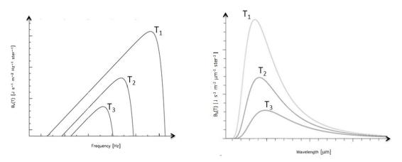
Radiance units should be correct, although I would accept either wavelength or wavenumber units (either the left or right plot). I do not need the actual temperatures on the curves or the numbers on the axes. Curves should not cross, and the hottest temperature, T1, should peak at shorter wavelengths (higher frequencies).
