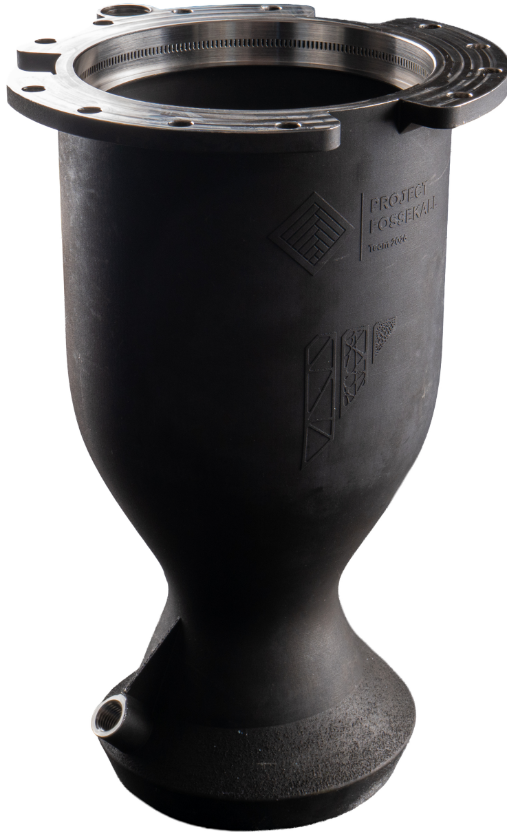
Figure 7.1: The P26 combustion chamber after printing, stress relieving and machining. Photo by Philip Draget, Propulse NTNU.
