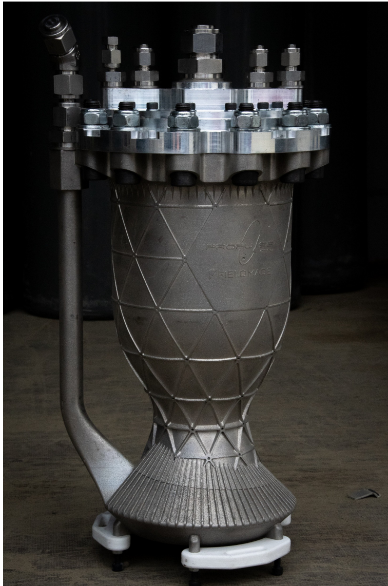
Figure 6.1: The P25 engine assembly, consisting of the combustion chamber, injector bulkhead, and injector plate (not visible). Photo by Propulse NTNU.
