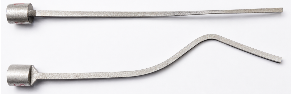
Figure 5.3: Cooling-channel test specimen manufactured for hydraulic assessment of the model: a single channel extracted from the P25 cooling-channel geometry and reprinted with the updated process parameters.
