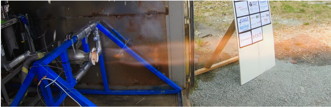
Figure 6.2: Static ground test of the P25 engine. The thermal analysis in this section is based on flight-test operating data, while the image is included to show the P25 test-firing configuration. Photo by Propulse NTNU.
