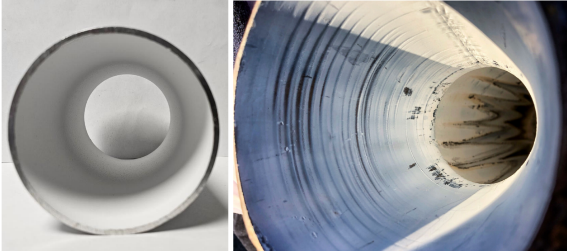
(a) Example of a TBC configuration dissimilar to the one used in this study. A 200 \mu\text{m} to 500 \mu\text{m} layer of ThermoHold ® is applied by atmospheric plasma spraying over a 50 \mu\text{m} nickel-based bond coat [1]. (b) Example of a TBC configuration closer to the one assumed in this study. A fine layer of silicon dioxide ( \text{SiO}_2 ) is formed in situ by combusting a fuel blend containing tetraethyl orthosilicate (TEOS), as demonstrated by Copenhagen Suborbitals [2]. The visible streak patterns result from the discrete injector orifices, rather than from a continuous annular distribution.
