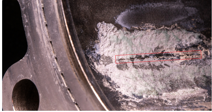
(b) Crack location after decommissioning
