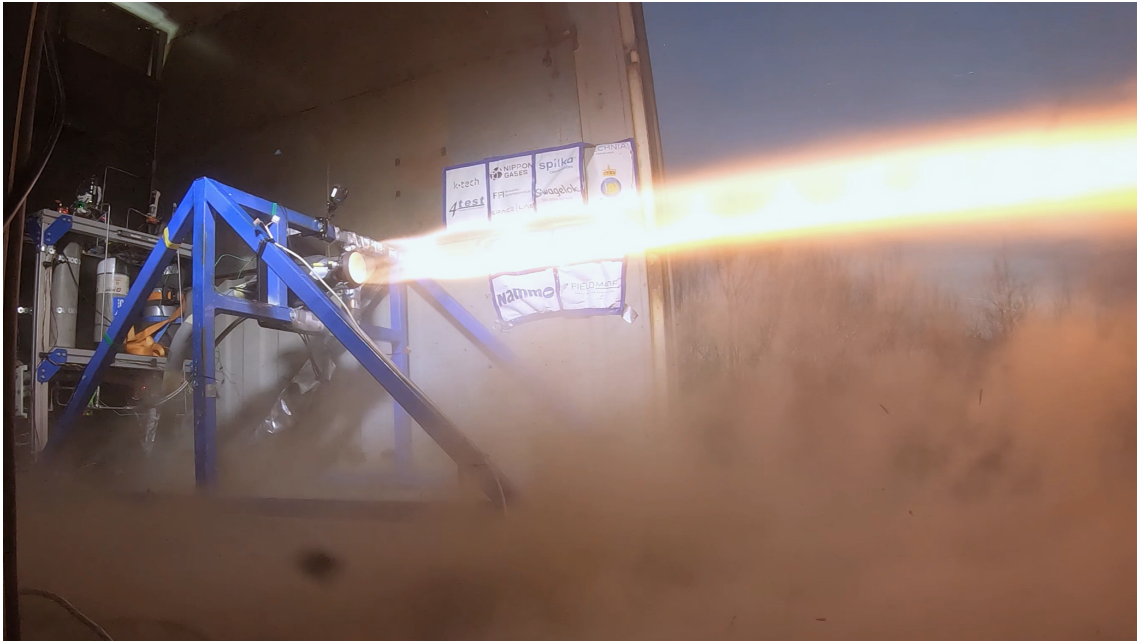
Figure 1.1: Static fire test of the P26 engine in a horizontal firing configuration. Photo by Philip Draget, Propulse NTNU.
