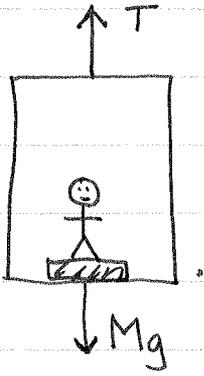
a)  $Ma = T - Mg \Rightarrow a = \frac{T - Mg}{M} = \frac{8300 - 750 \cdot 9.8}{750} \text{ m/s}^2 \approx \underline{\underline{1.3 \text{ m/s}^2}}$
