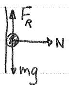
$$N = m\omega^2 r \quad \text{og} \quad F_R = F_R^{\max} = \mu N = mg$$
